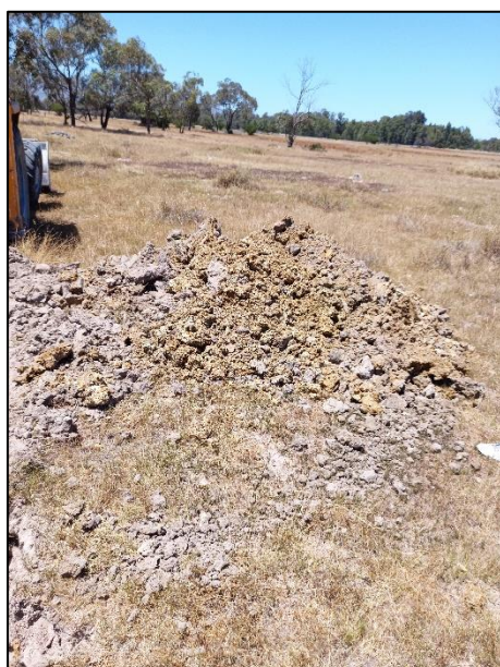
Figure 9-1: Residual shale excavation spoil adjacent to trial pit TP7 (left) and residual shale excavation spoil adjacent to trial pit TP25
