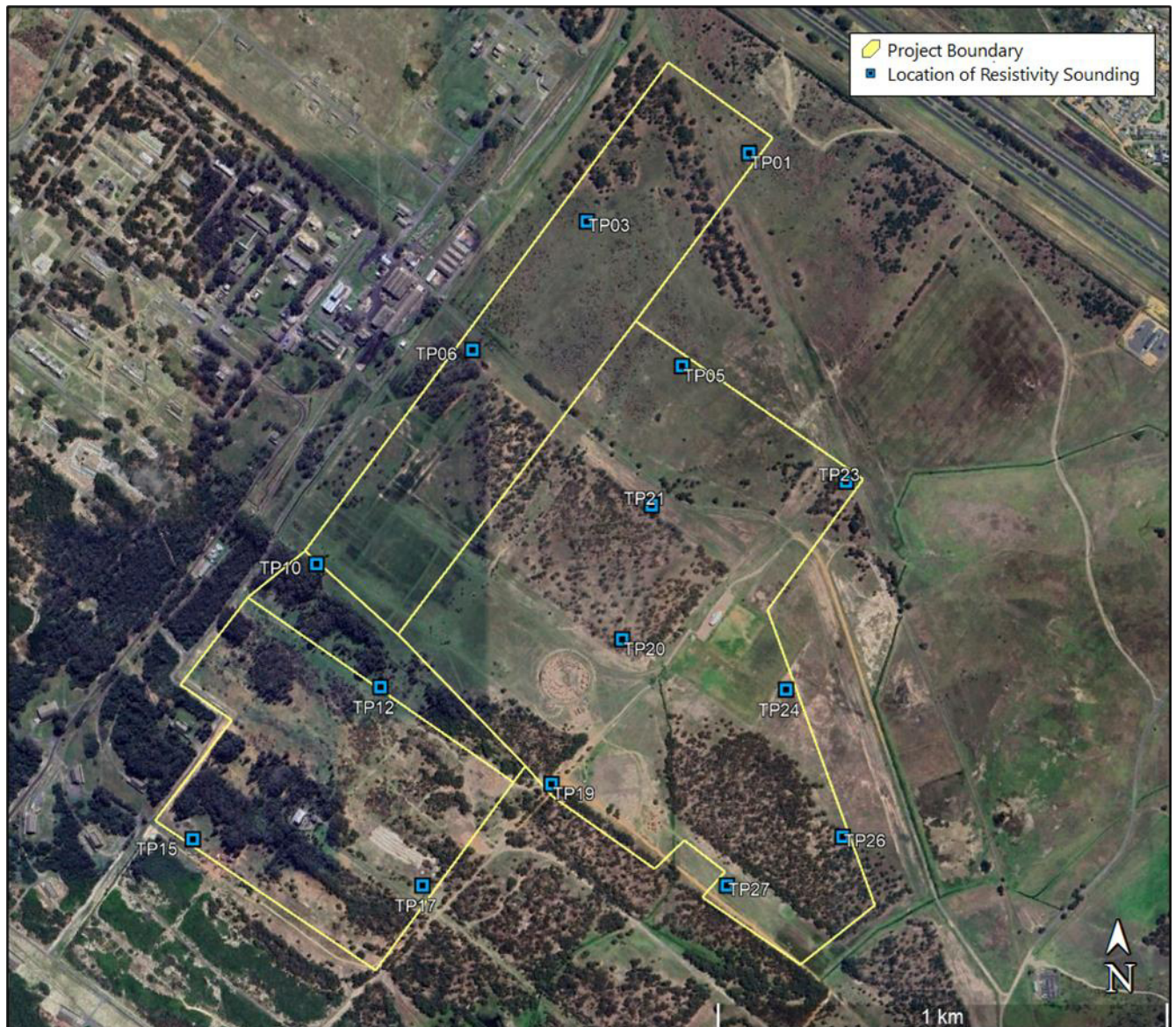
Figure 2: Site Plan Showing Sounding Test Positions
