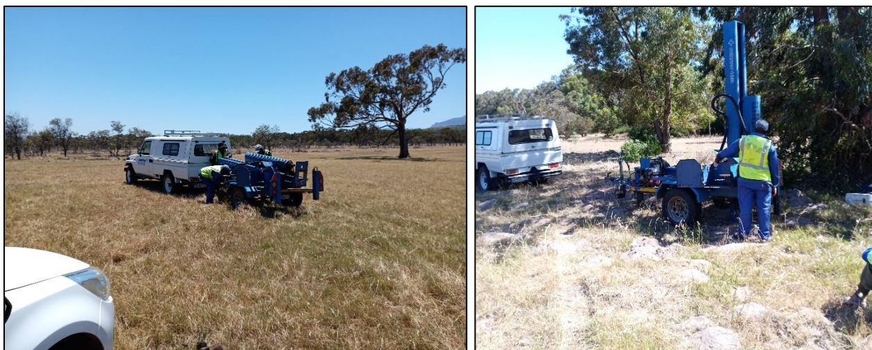
Figure 6-1: DPSH rig setup (left) and DPSH testing at Paardevlei Solar PV Farm site (right)
