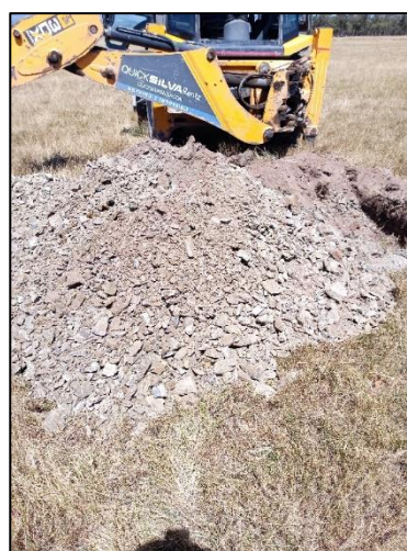
Figure 7-4: Hardpan calcrete (left) and weathered shale bedrock spoil material (right)
