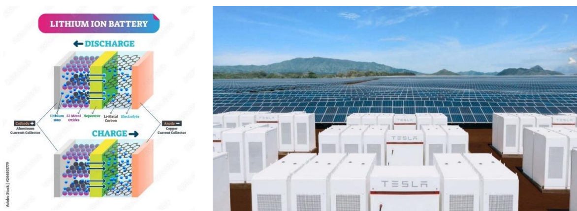
Figure 23: Li-ion battery system scheme and example of a Tesla Li-ion BESS system in utility-scale solar PV plant
