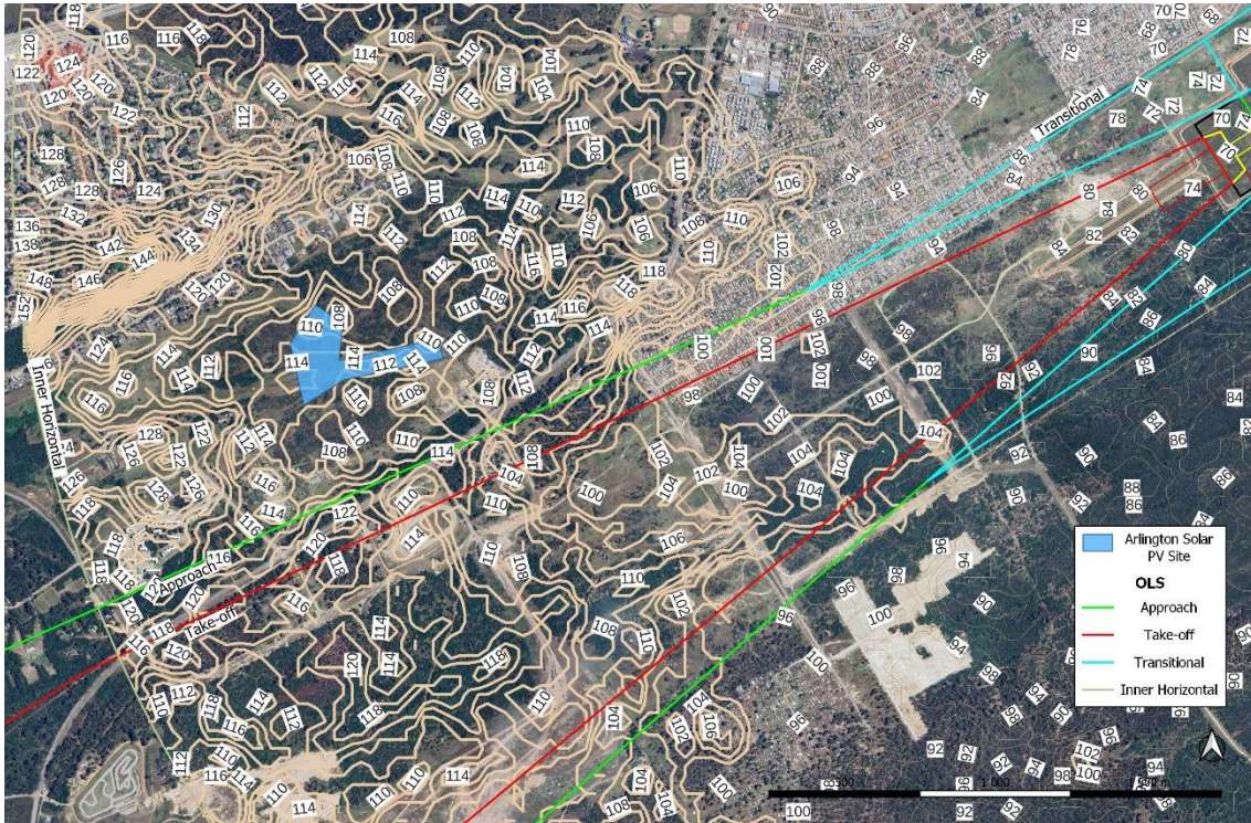
Fig 8: SRTM data showing terrain above 101m (AMSL)
