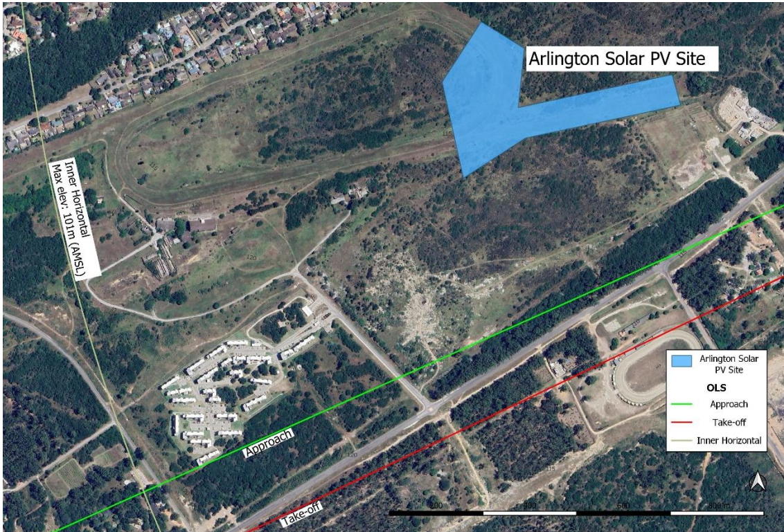
Fig 6: Inner Horizontal max elevation 101m (AMSL)
