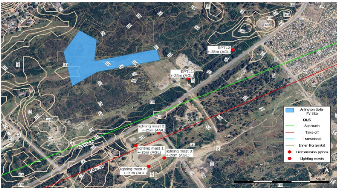
Figure 77: AIP and other obstacles within the vicinity of the proposed PV development
