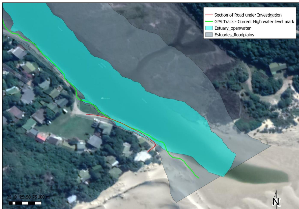
Figure 2: Proposed position (red line) of the erosion protection feature in relation to current inundation levels measured October 2018 (green line)
